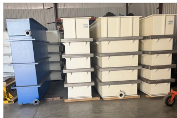
New polypropylene and steel process tanks, interiors unused.
