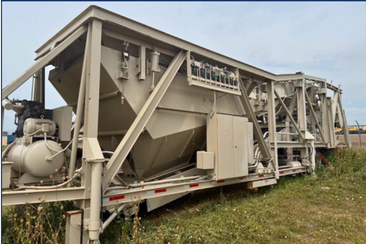
CON-E-CO AllPro Super Portable 12 CY Central Mix Concrete Plant, SN C5093
