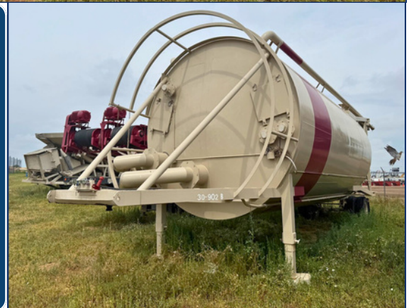
CON-E-CO AllPro Super Portable 12 CY Central Mix Concrete Plant, SN C5093
